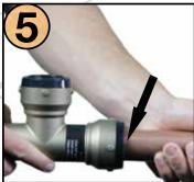
Connection is complete when pipe is fully inserted with depth insertion marked on pipe is still visible at the head of the fitting.
